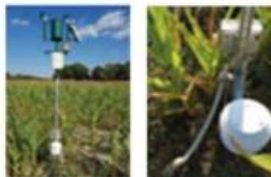
air temperature, humidity, wind speed, precipitation and global radiation
