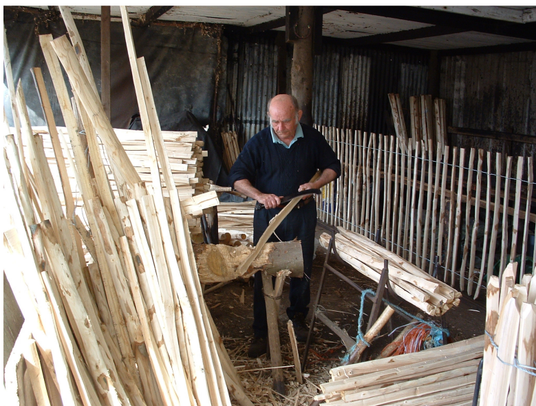
An entrepreneur making traditional chestnut paling fencing in the UK
